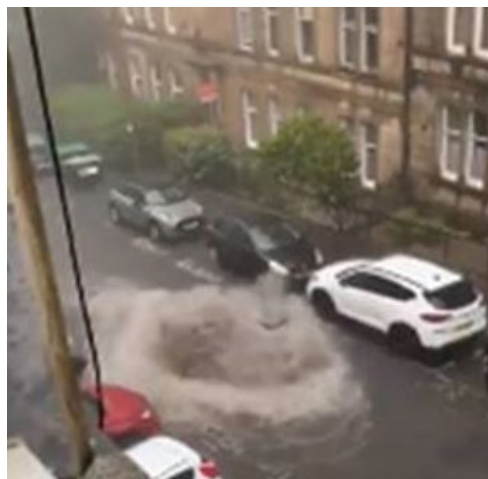
Example: Surcharging Sewer System at Capacity
